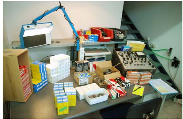
Each and every vacuum tube we use goes through a series of tests which partly performed on our vintage HICKOK MODEL 539C MUTUAL CONDUCTANCE TUBE TESTER which allows us to match between vacuum tubes and spec performance.
