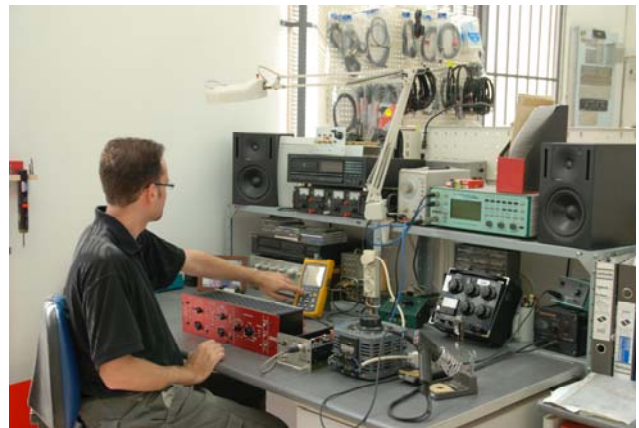
This is our final assembling stage in which we test each and every instrument we manufacture for spec performance and perform a "burn in" test for tube instruments.
