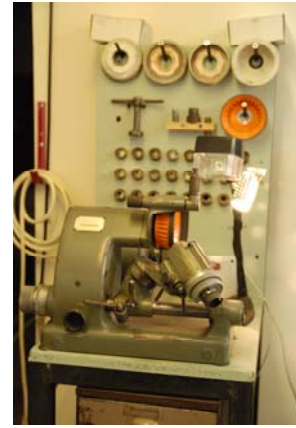
This is our 60 yrs` old DECKEL FINEMECHANIK leap cutter grinding machine which we use for our grinding CNC cutters.
