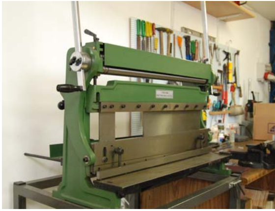
This is a combined metal 3-IN-1/760mm SHEAR PRESS BRAKE & SLIP ROLL machine which we use on fabricating small metal parts.
