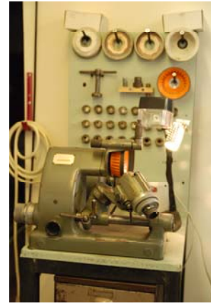
This is our 60 yrs` old DECKEL FINEMECHNIK leap cutter grinding machine which we use for our grinding CNC cutters.
